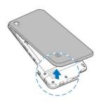
Hold the nano-SIM card with its cut corner oriented as shown and slip it into the card holder.
