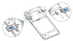
Hold your microSDXC card with the metal contacts facing down and slide it into the microSDXC card slot.
